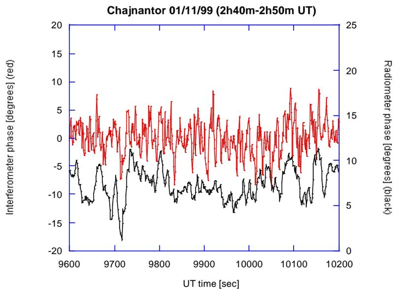
**Phase variation measured with radiometer (red curve) compared with ambient temperature (lower, black curve)**
