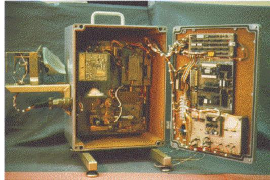
Figure 6 225 GHz tipping radiometer.
