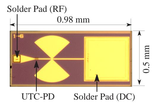
Fig. 2 Photograph of a UTC-PD chip.
