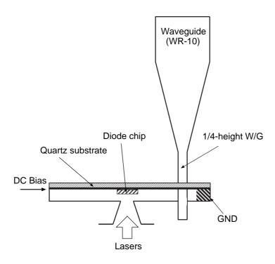
Fig. 4 Schematic of a photomixer mount.
