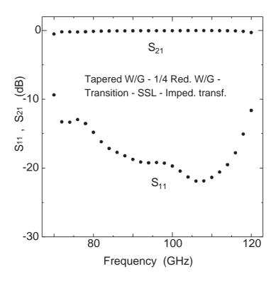
Fig. 5 Predicted performance of the waveguide-stripline transition.
