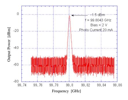
Fig. 8 Spectrum of photomixer output at  $\sim$ 100 GHz.
