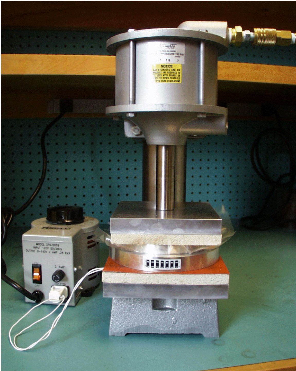
Figure 9. Photograph of the assembled window press. The Variac and heating pad are used to increase the temperature of the jig and so decrease the curing time of the epoxy. Note the thin film thermometer on the lower half of the jig.
