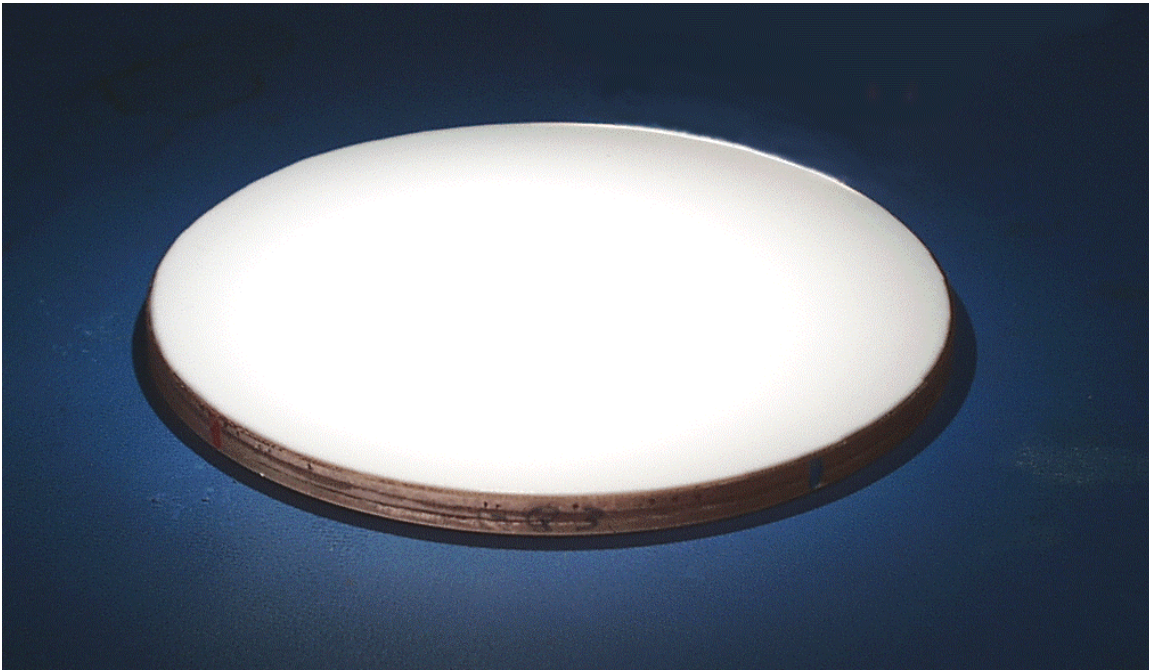
Figure 10. A nearly completed 4.5" diameter, three-layer window for the VLBA. The outer surfaces are PTFE, which has not yet been trimmed for the O-ring seal.
