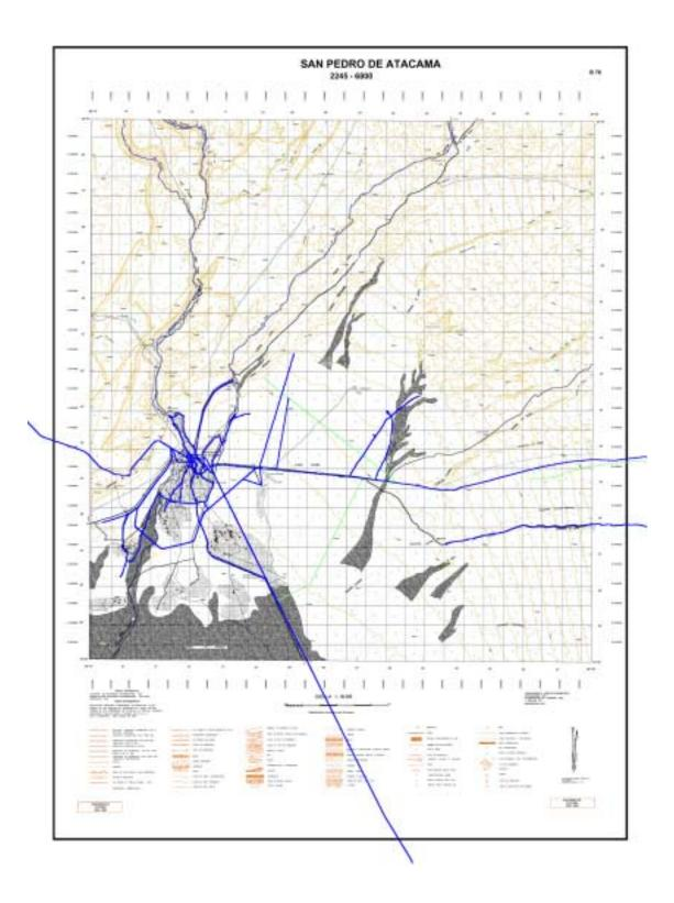
Figure 5: Loci of roads and trails (blue lines) and pipelines (green lines) overlaid on 1:50,000 topographic map of San Pedro de Atacama [11]. The map covers  $0.25^{\circ} \times 0.25^{\circ}$  (equivalent to about 25 km  $\times$  28 km) area centered at 22.875° S and 68.125° W. Grids are in UTM Zone 19 easting and northing spaced by 1 km. Contour spacing is 50 m.
