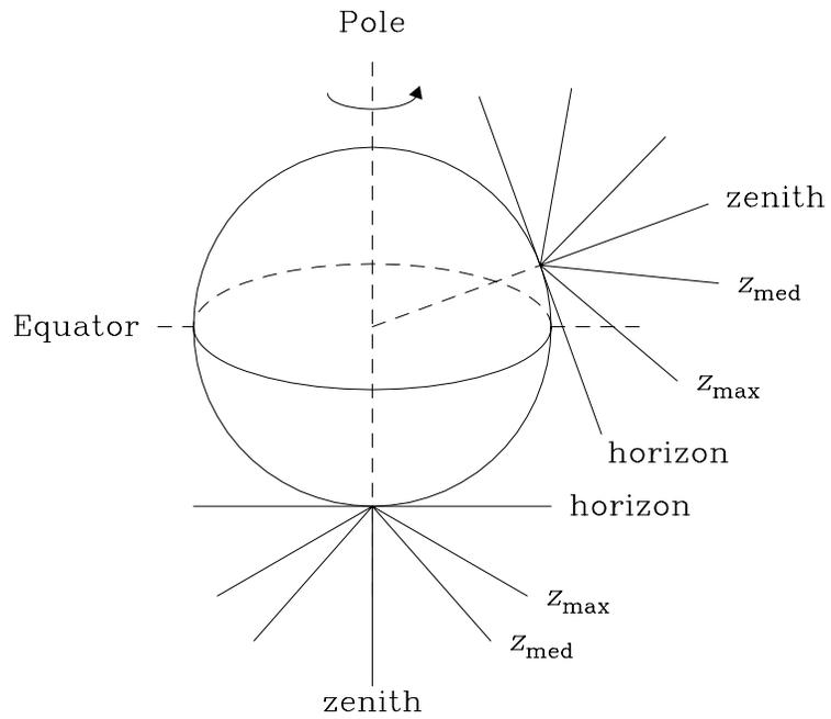
Figure 1: Observing geometry at tropical ( $20^\circ$  latitude) and polar sites. The median zenith angle ( $z_{\text{med}}$ ) is shown for observations near meridian transit with  $z_{\max} = 60^\circ$ .
