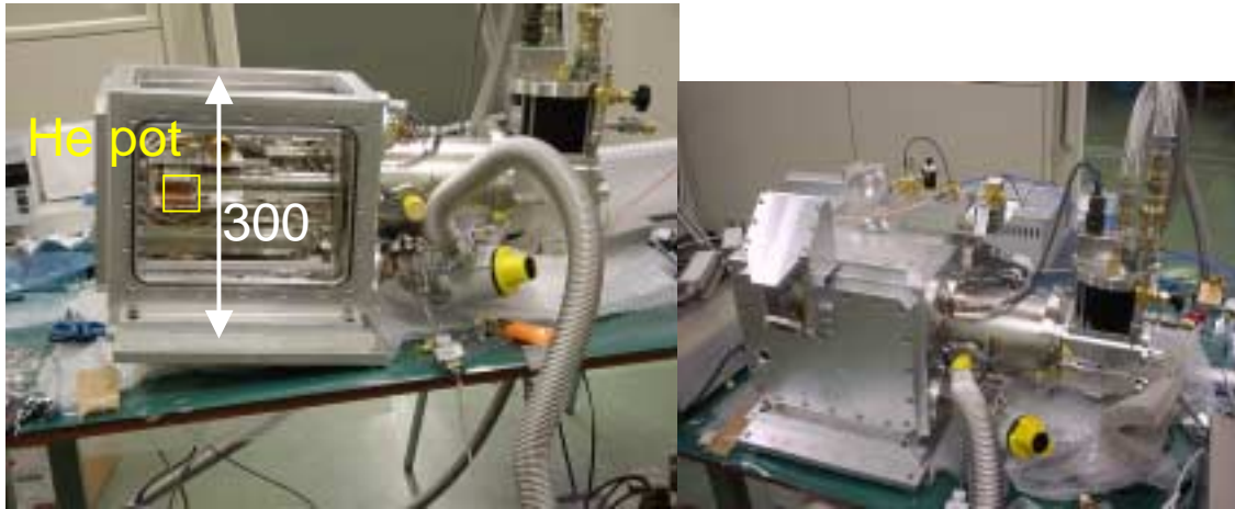
Figure 3: Photographs of the ASTE 350 GHz receiver. The cryocooler is Sumitomo RDK408DA. The cryocooler employs a He pot made of copper on the head of the 4K stage.
