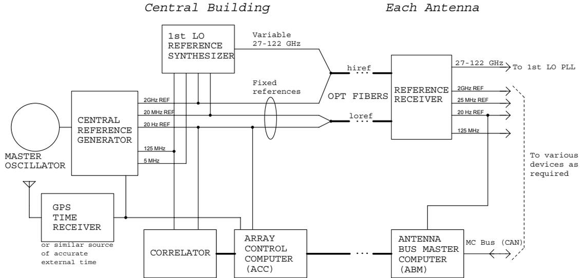
Figure 1: Simplified block diagram of the time distribution hardware.
