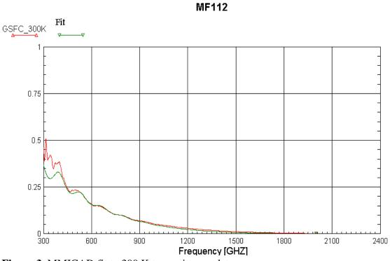
Figure 3 MMICAD fit to 300 K transmittance data.
