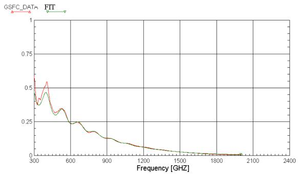
Figure 4 MMICAD fit to 5 K transmittance data
