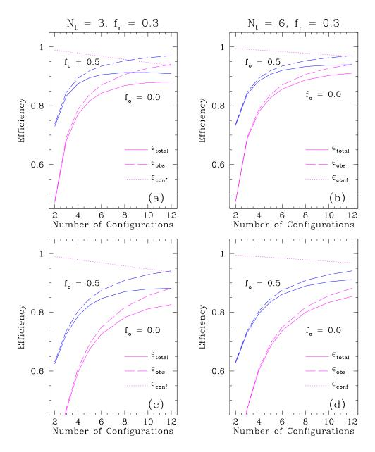
Figure 6: Effects of increasing the number of transporters and move crew for  $N_t = 3$  and  $N_t = 6$  with  $f_r = 0.3$ . The main difference is in the configuration efficiency,  $\epsilon_{conf}$ , which scales as  $1/N_t$ . As in Figures 4 & 5, (a) & (b) are for p = 0.5 and (c) & (d) are for p = 1.
