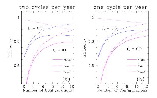
Figure 1: A comparison of the array efficiency between one full configuration cycle per year and two configuration cycles per year. The cases considered here are essentially the same as in Figures 1&2 of Holdaway (1998). The main difference is in the reconfiguration efficiency (dotted line), and the monetary cost comparison is given in Table 1.
